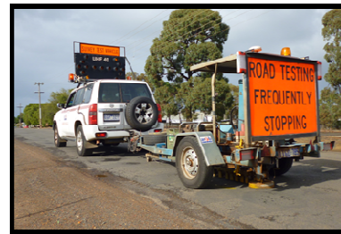
(Pictured above: road pavement testing in progress)
