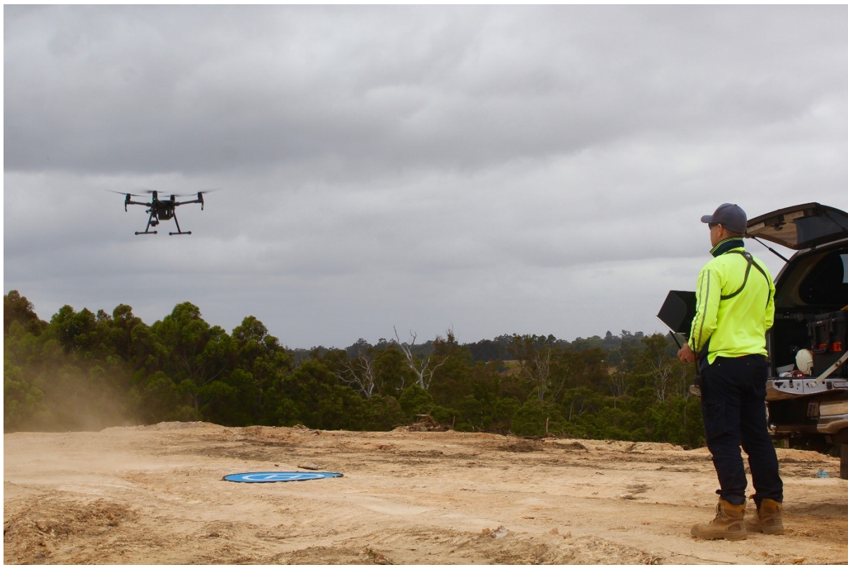
The surveying contractor used a drone to carry out an aerial volumetric survey of the landfill.
