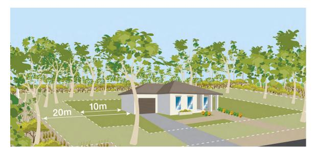
Figure 5: Measuring zones around a building
