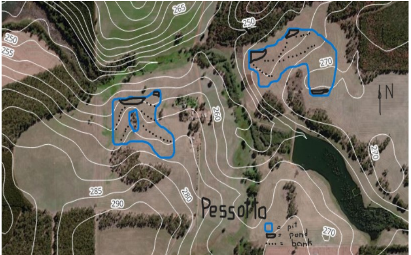
Plan C: Proposed gravel extraction areas showing proposed water retention ponds and temporary contour bunds (banks) at 148 Whim Landing Road.
